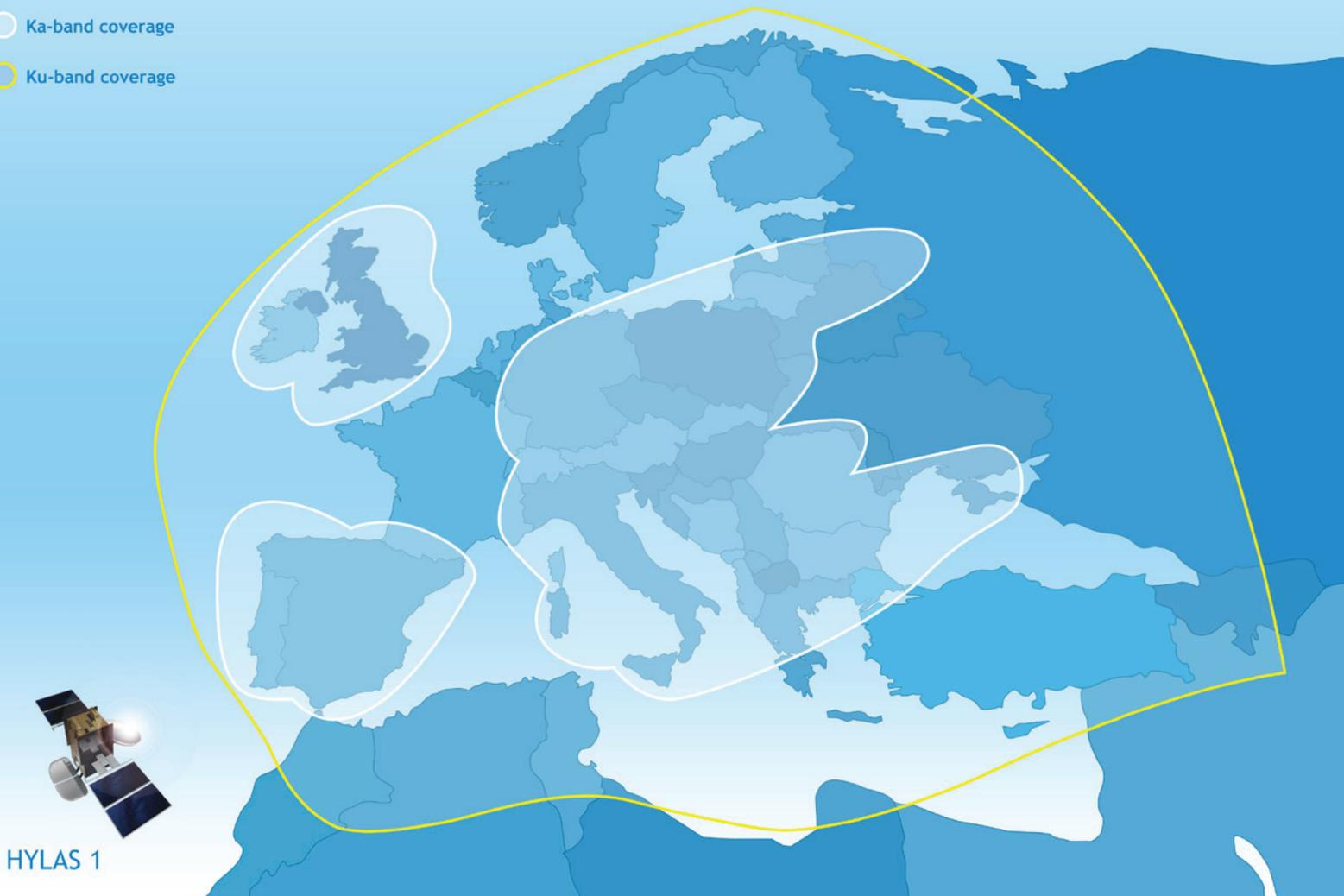
**HYLAS 1 IS AVANTI'S FIRST BROADBAND SATELLITE AND USES THE LATEST KA-BAND TECHNOLOGY** to deliver high speed, two-way data services across Europe. It has a unique flexible payload which enables Avanti to change the bandwidth of its 8 Ka-band beams, whilst in orbit, to maximise satellite efficiency. HYLAS 1 is complemented by a Ku-band broadcast capability.
