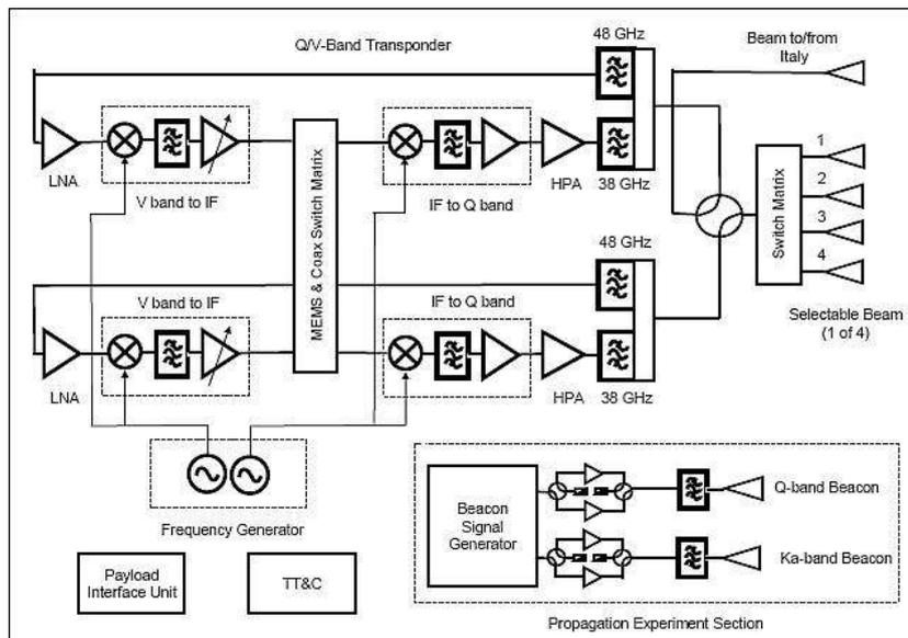
Figure 25: Alphasat Q/V-band payloads block diagram including propagation section (image credit: ASI)
