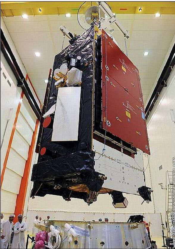
Figure 12: Photo of the Alphasat being lowered onto the Arianespace flight adapter in Kourou (image credit: ESA) [21](#)
