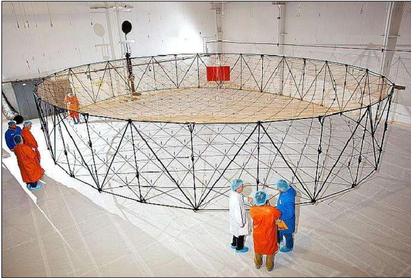
Figure 18: Photo of the deployed AstroMesh reflector (image credit: Astro Aerospace)
