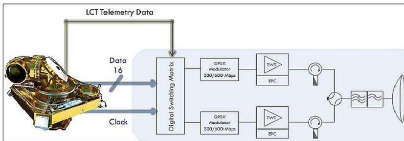
Figure 23: Alphasat data relay payload (image credit: Tesat) [45](#)**Q/V-band transponder payload (TDP5) / Aldo Paraboni Payload:**
