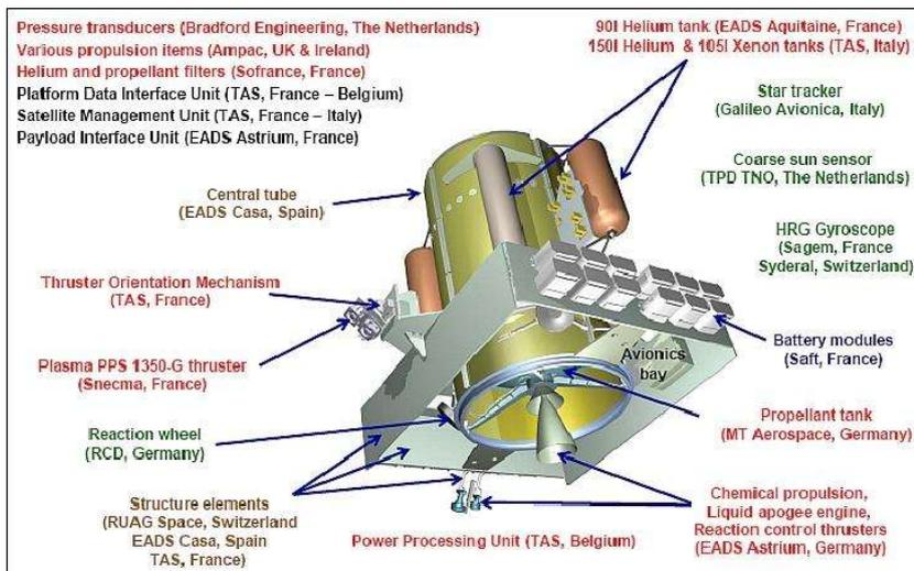
Figure 4: Allocation of Service Module element manufacturing to European companies (image credit: CNES)
