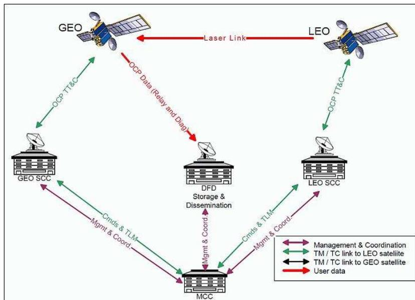
Figure 41: Schematic view of the TDP1 GEO relay system (image credit: DLR/GSOC)
