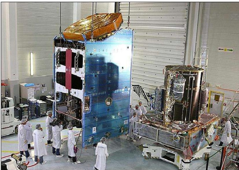
Figure 3: Photo of the Alphasat service module (right) and Alphasat repeater module stand side by side before the mating procedure at Astrium SAS (image credit: Astrium)
