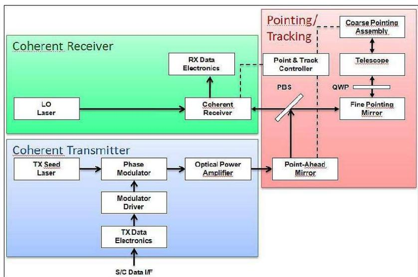
**Figure 21: Block diagram of the LCT instrument** (image credit: Tesat Spacecom)
