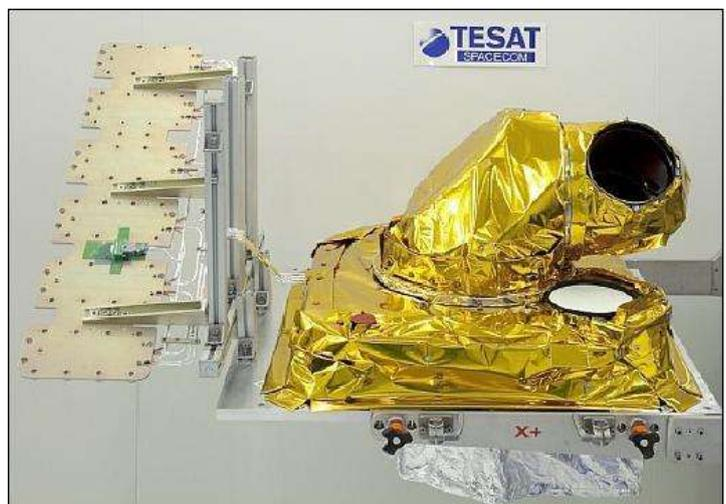
**Figure 22: Alphasat LCT, equipped with MLI, with an Alphasat specific thermal Interface, mounted in its**
