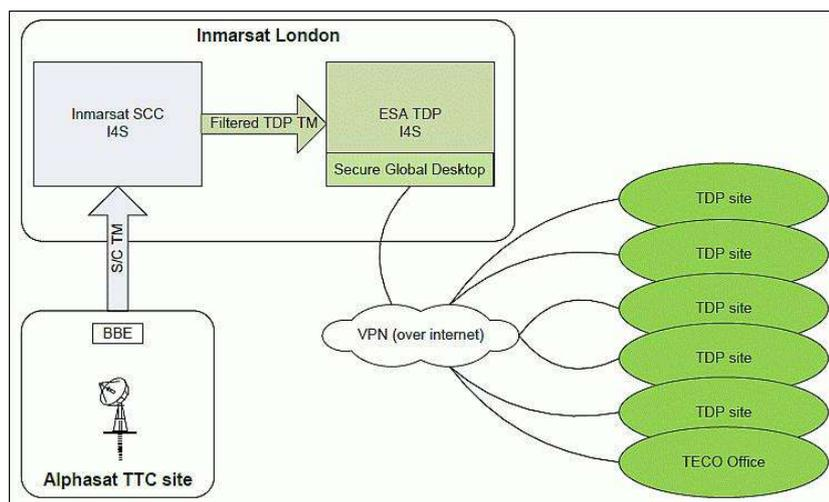
Figure 39: ESA (TECO) TDP I4S system architecture (image credit: ESA, Inmarsat)
