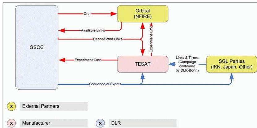
Figure 42: TerraSAR-X LCT operations concept (image credit: DLR/GSOC)
