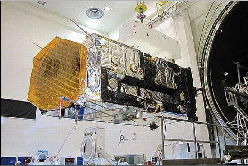
Figure 11: The Alphasat spacecraft entering the thermal vacuum chamber in Toulouse in late November 2012 (image credit: Intespace) [19](#) [20](#)
