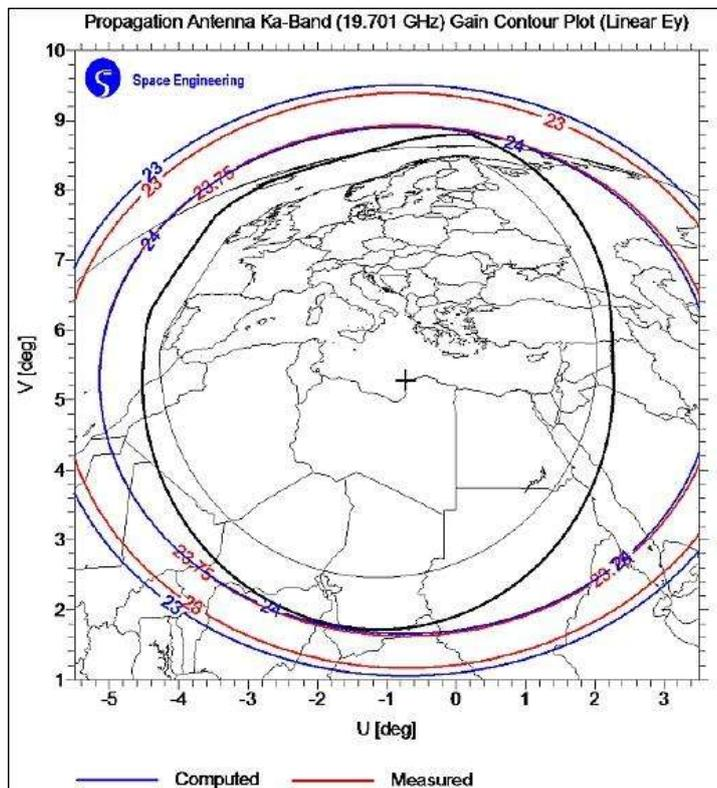
Figure 30: Alphasat TDP5 beacon coverage of the Ka-band, 19.701 GHz [56](#)
