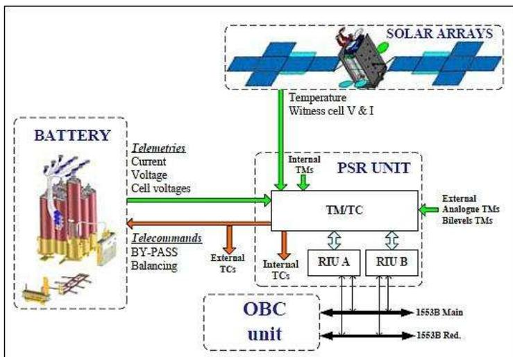
Figure 9: EPS TM/TC block diagram (image credit: Astrium SAS)
