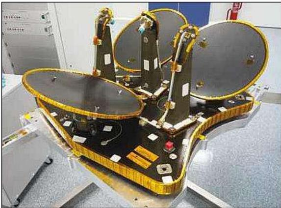
Figure 24: Photo of the Q/V-band communication repeater - also referred to as QVCA (image credit: TAS-I)
