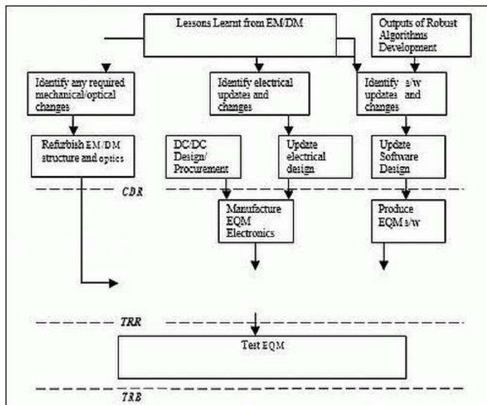
Figure 33: ASTRO-APS Star Tracker qualification project plan (image credit: Jena-Optronik, ESA)
