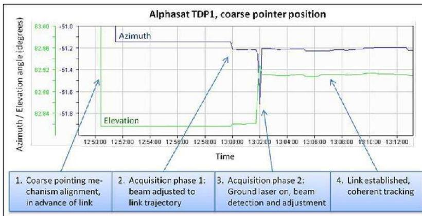
Figure 14: Beam steering mechanism position during link acquisition (image credit: Tesat)
