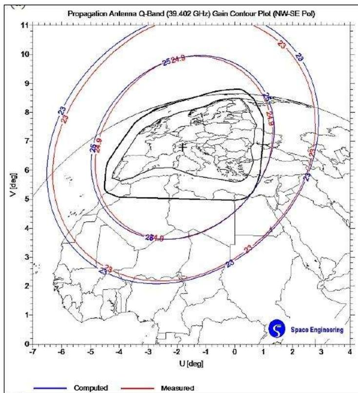
Figure 31: Alphasat TDP5 beacon coverage of the Q-band, 39.402 GHz
