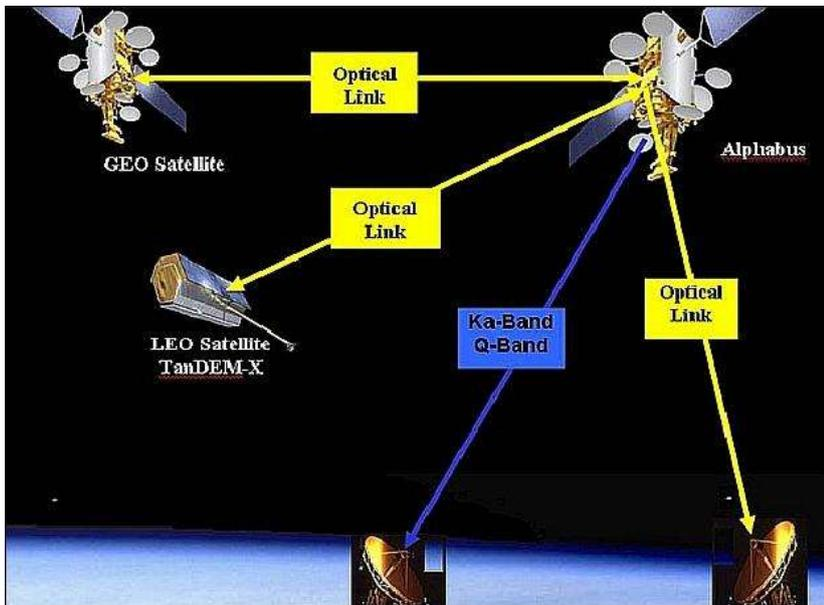
Figure 1: Illustration of communications links with Alphasat I-XL (image credit: ESA, TAS)
