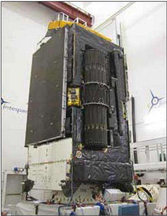
Figure 10: Photo of Alphasat after the mechanical test campaign in August 2011 (image credit: ESA)
