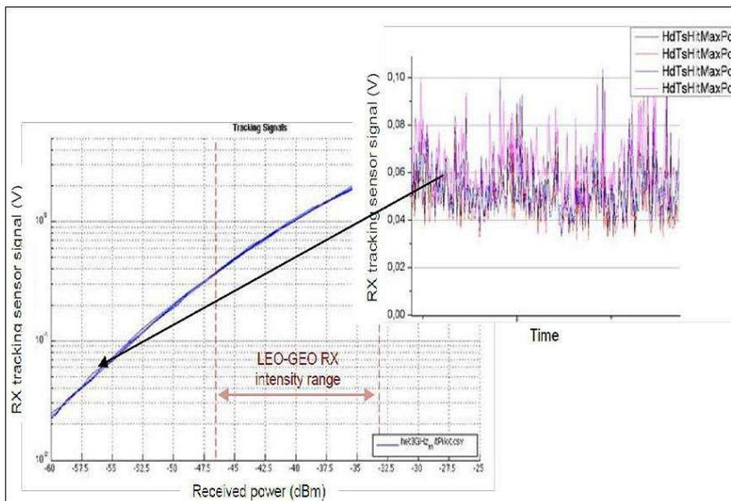
Figure 15: Coherent tracking at GEO-ground RX signal strength (inlay), much below LEO-GEO RX intensity (image credit: Tesat, Ref. 44)
