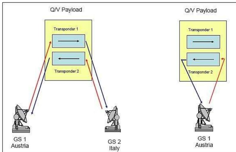
Figure 26: Modes of operations: Cross-strap mode (left), Loop-back mode (right), image credit: TU Graz
