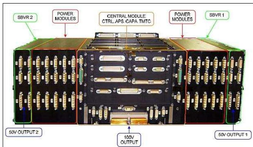
Figure 7: The PSR100V unit with 10 PMs and 2 SBVRs (image credit: Astrium SAS)
