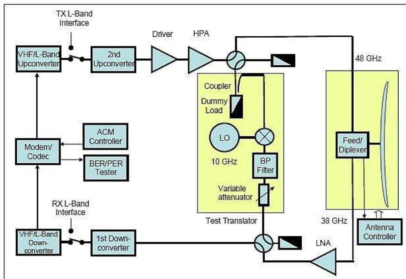
Figure 27: Block diagram of the Alphasat ground terminal (image credit: TU Graz)
