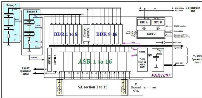
Figure 8: Functional block diagram of PSR100V (image credit: Astrium SAS)
