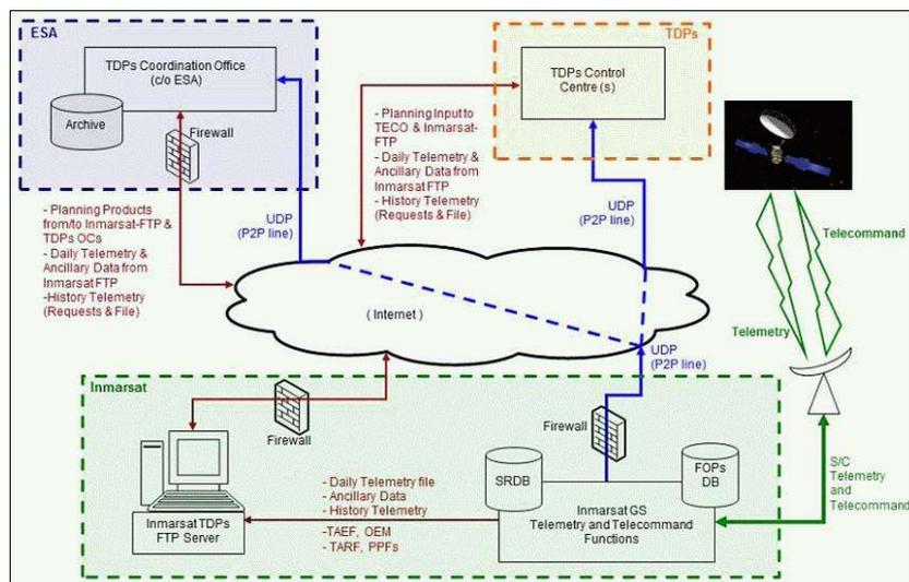
Figure 37: TDPs Monitoring and Control GS topological architecture (image credit: ESA, Inmarsat)
