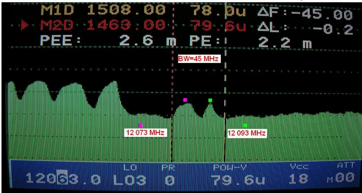
Chinasat 9 at 92,2° E - KU Asian SPOT : two more none locked carriers 12 073 / 12 093 in spectrum detail
