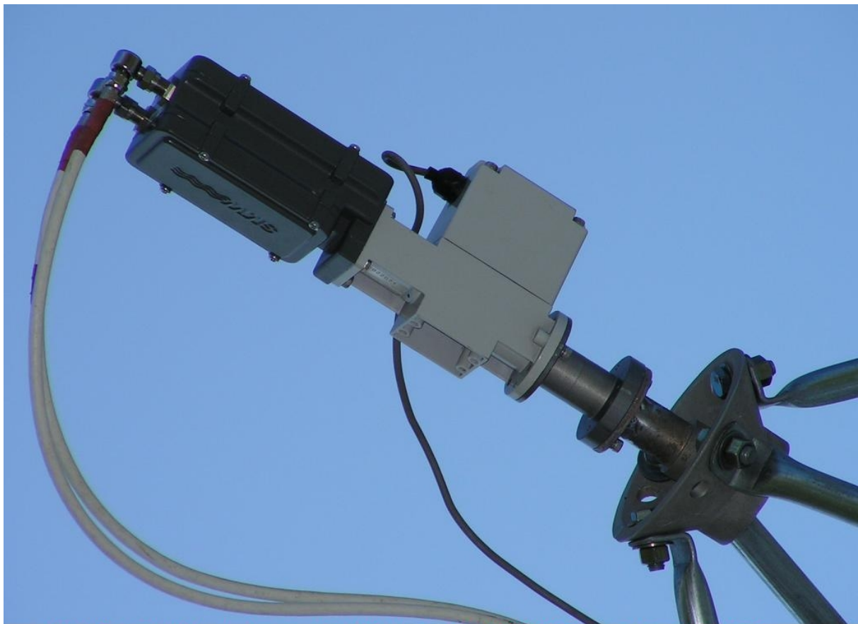
dxsatcs HF assembly for best vector conversion (LC to V) with minimal IN-OUT VSWR ratio and maximal gain transfer
